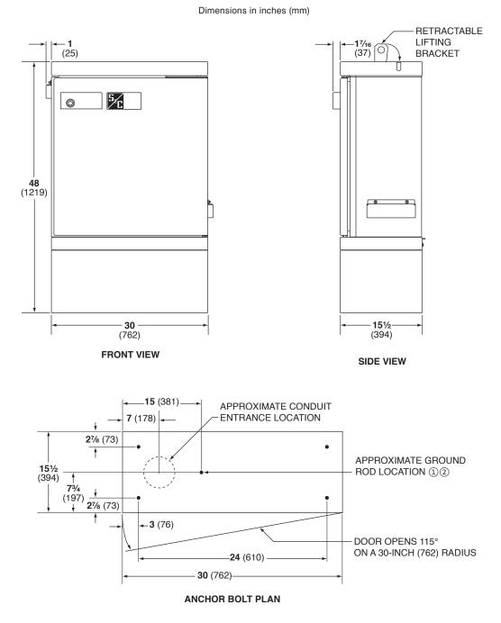
① Attach earth ground cable between the ground lug inside the low-voltage enclosure and the ground rod using copper cable of 4/0 or greater and less than 10 feet (305 cm) in length.
