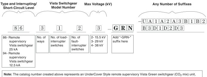
**Note:** The catalog number created above represents an UnderCover Style remote supervisory Vista Green switchgear ( $CO_2$  mix) unit, 25 kA, with a total of three ways that includes one load-interrupter switch and two fault-interrupter switches for a 29-kV application. All three ways will have the motor operator package, three-phase current sensing, and three-phase voltage sensing.
