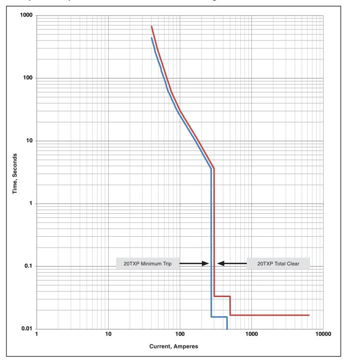
20-Ampere TXP-Speed TCC Curve with Definite Times at High Current
