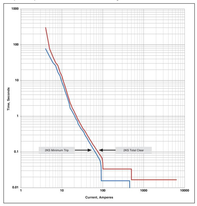
2-Ampere KS-Speed TCC Curve with Definite Times at High Current
