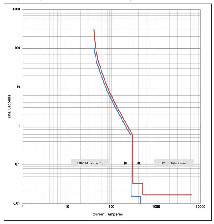
20-Ampere KS-Speed TCC Curve with Definite Times at High Current
