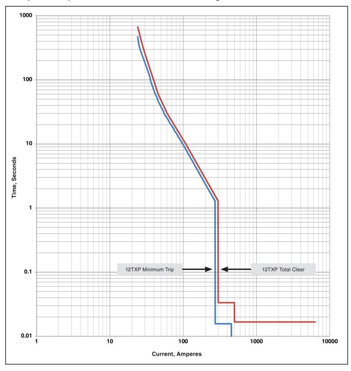
12-Ampere TXP-Speed TCC Curve with Definite Times at High Current
