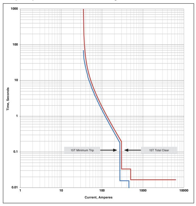
15-Ampere T-Speed TCC Curve with Definite Times at High Current
