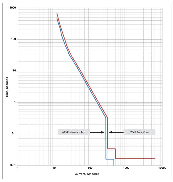
6-Ampere TXP-Speed TCC Curve with Definite Times at High Current
