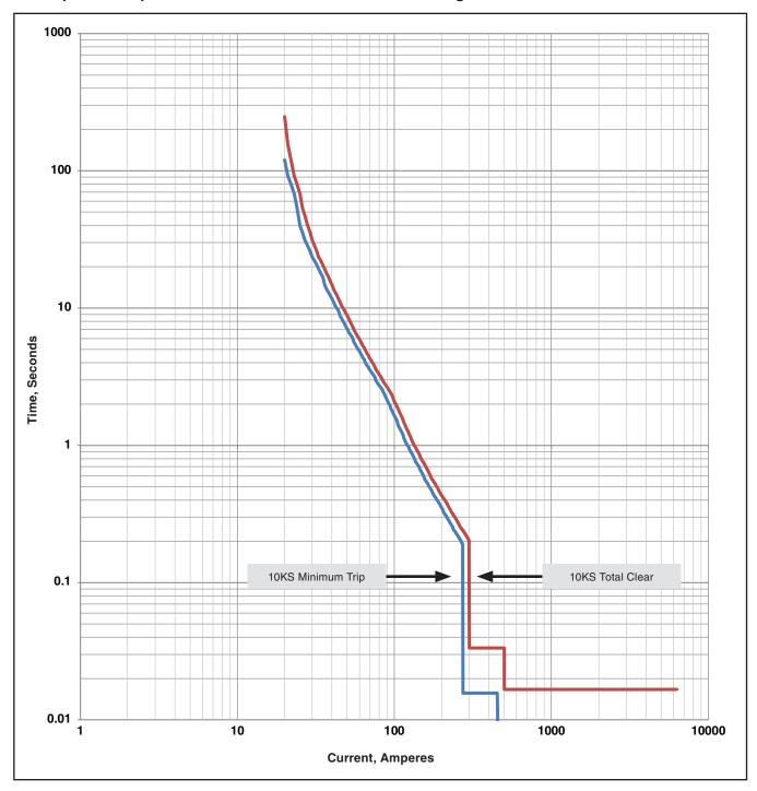
10-Ampere KS-Speed TCC Curve with Definite Times at High Current
