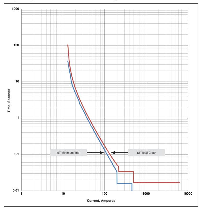
6-Ampere T-Speed TCC Curve with Definite Times at High Current
