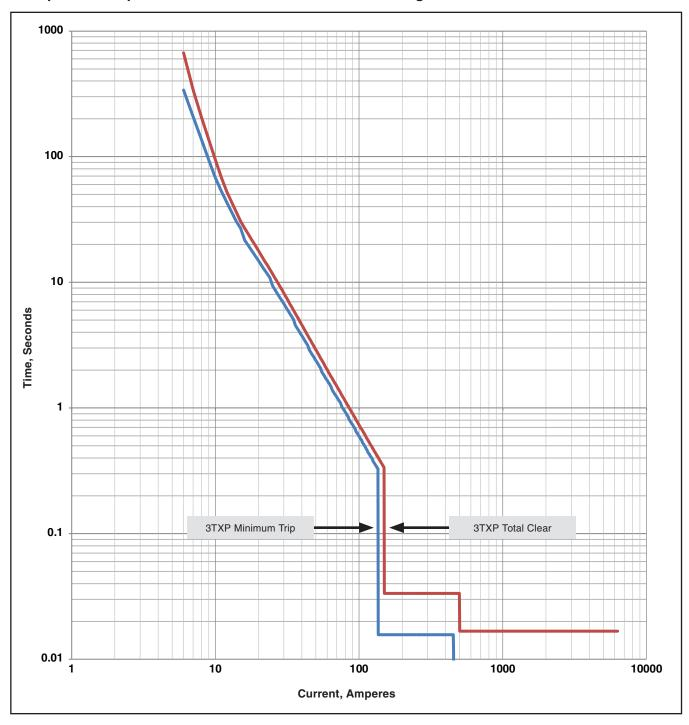
3-Ampere TXP-Speed TCC Curve with Definite Times at High Current
