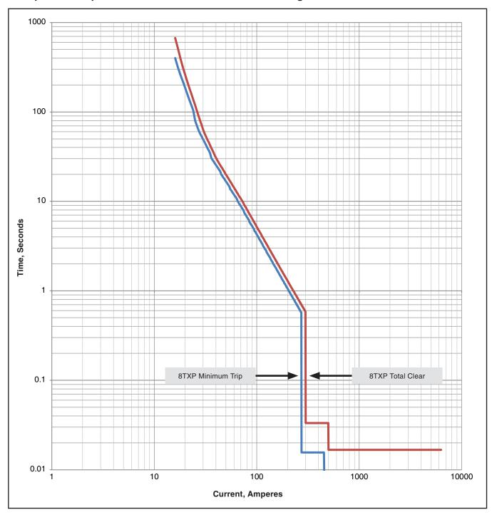
8-Ampere TXP-Speed TCC Curve with Definite Times at High Current
